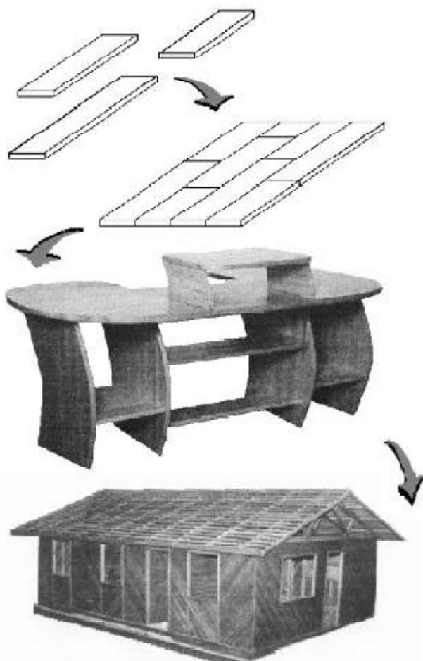
**Figure 2.** Process design of assembly of the glued wood panels and examples of the use of glued eucalypt wood panels at the furniture industry and at the civil engineering (projects developed at the IPT – Institute of Technological Researches of the São Paulo State).
