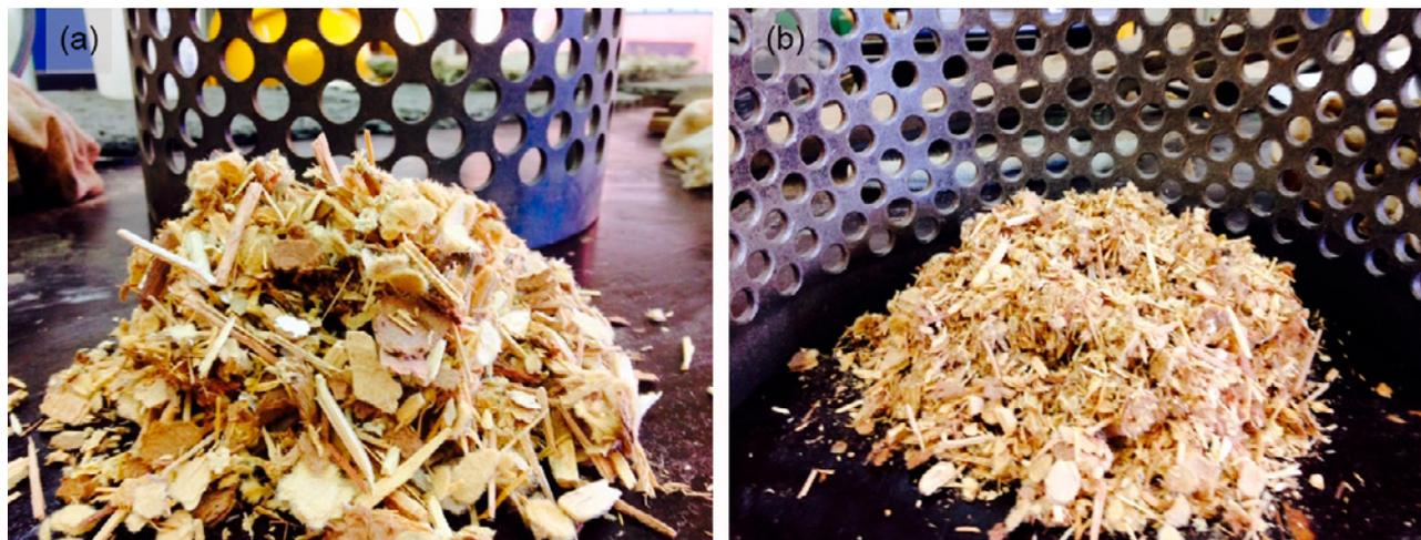
**Figure 1.** Hammer mill sieves with respective furniture disposal particles: (a) 18 mm mesh and (b) 12 mm mesh.
