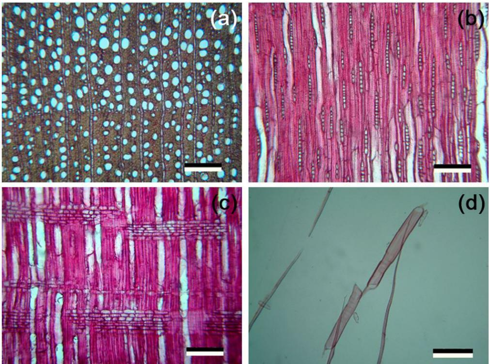
**Figure 2.** Histological sections of the *A. pyriformium* wood collected in site 1 (S1) and site 2 (S2), Sergipe state, Brazil: (a) transversal plane, bar; (b) tangential longitudinal plane; (c) radial longitudinal; (d) macerated; Bar = 200  $\mu$ m.
