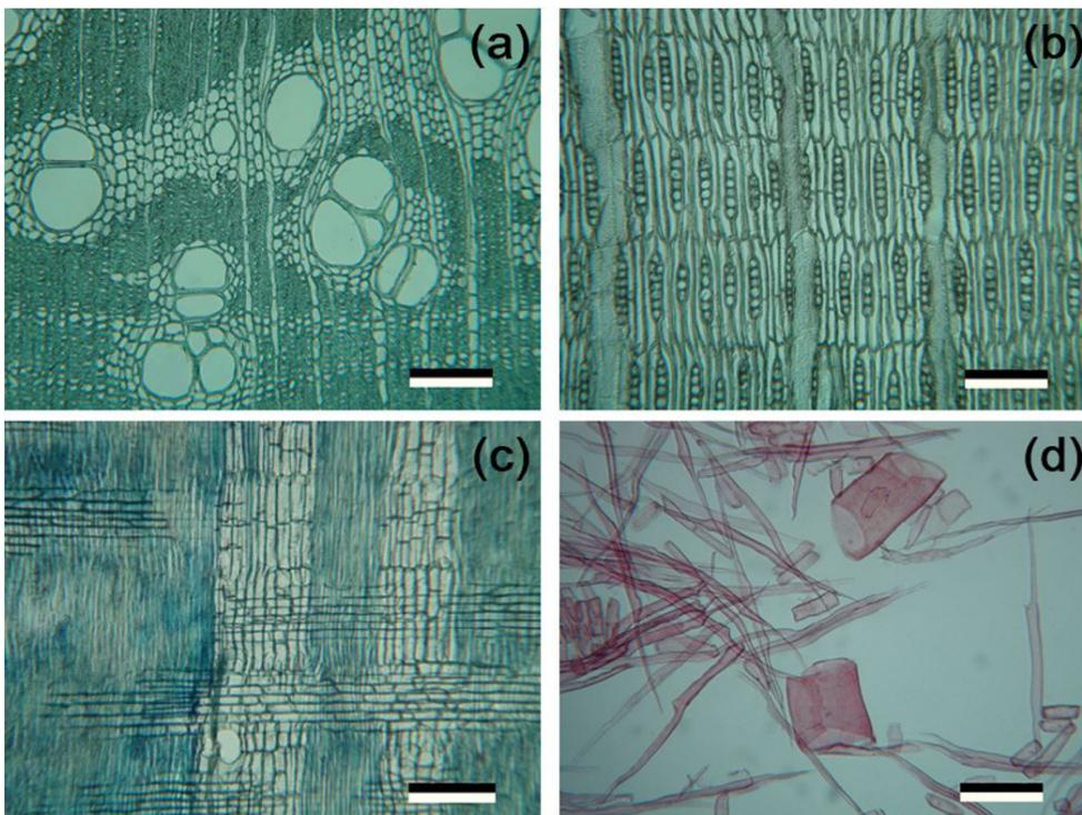
**Figure 4.** Histological sections of the *T. aurea* wood collected in site 1 (S1) and site 2 (S2), Sergipe state, Brazil: (a) transversal plane, bar; (b) tangential longitudinal plane; (c) radial longitudinal; (d) macerated; Bar = 200  $\mu\text{m}$ .
