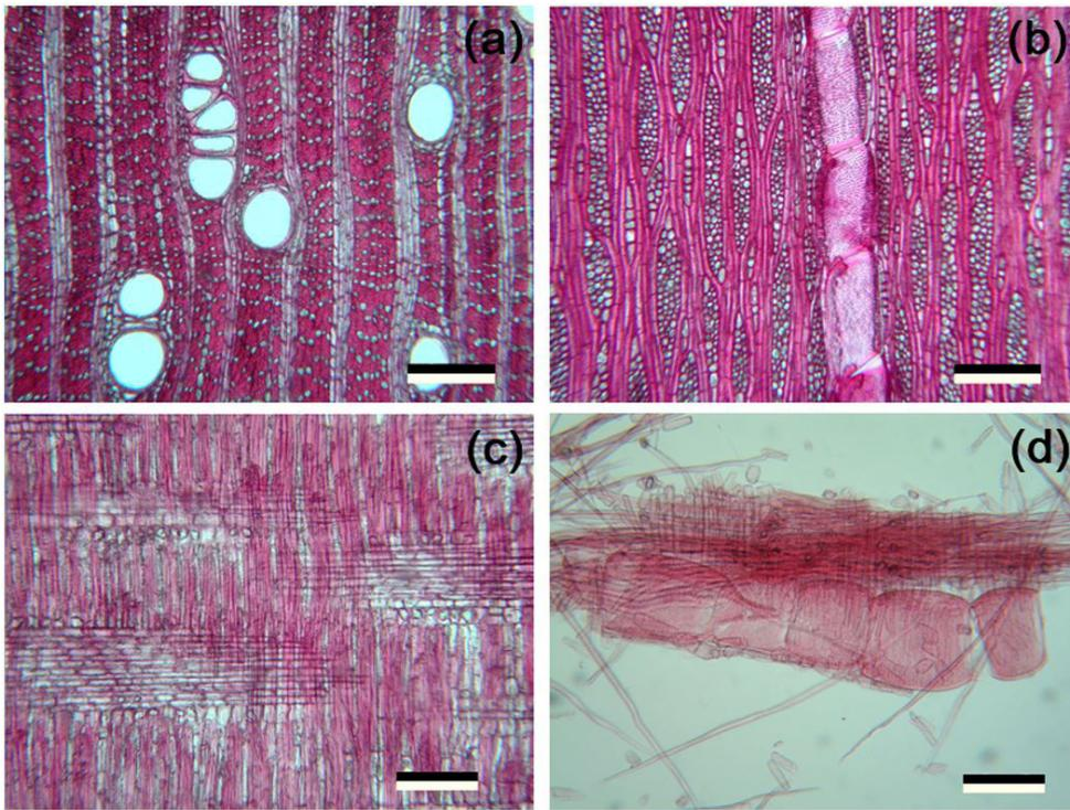
**Figure 3.** Histological sections of the *Z. joazeiro* wood collected in site 1 (S1) and site 2 (S2), Sergipe state, Brazil: (a) transversal plane, bar; (b) tangential longitudinal plane; (c) radial longitudinal; (d) macerated; Bar = 200  $\mu\text{m}$ .
