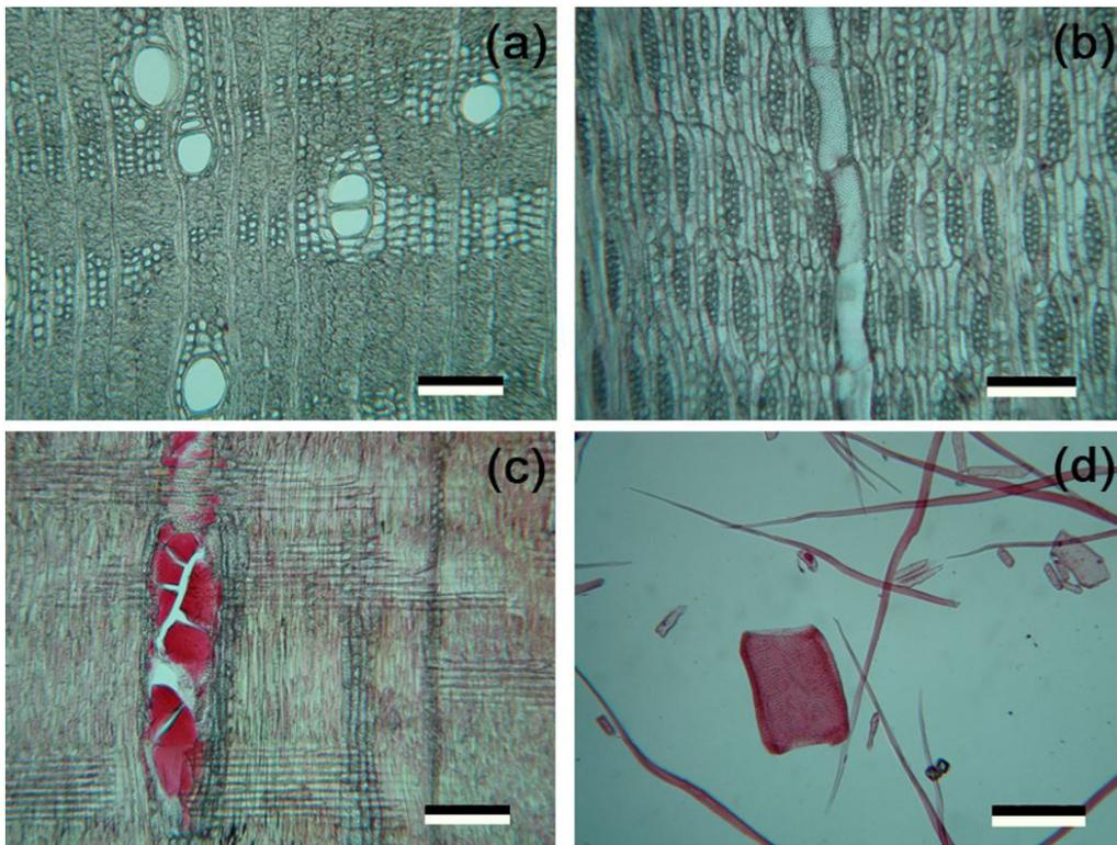
**Figure 5.** Histological sections of the *L. ferrea* wood collected in site 1 (S1) and site 2 (S2), Sergipe state, Brazil: (a) transversal plane, bar; (b) tangential longitudinal plane; (c) radial longitudinal; (d) macerated; Bar = 200  $\mu\text{m}$ .
