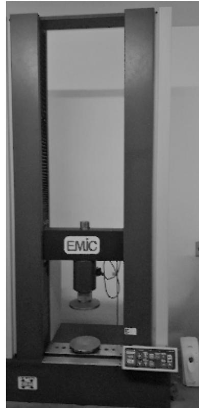
**Figure 2.** Universal testing machine used to evaluate mechanical resistance of the panels.
