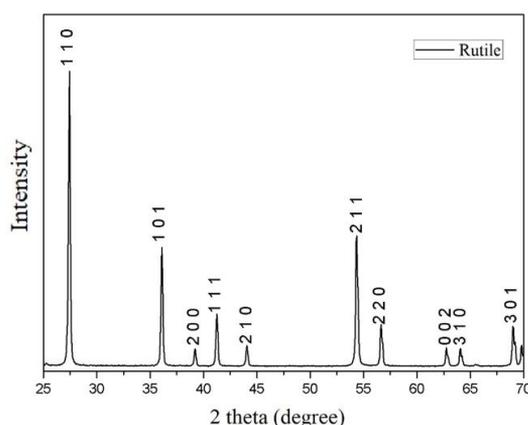
**Figure 1.** X-Ray Diffractogram of the commercial  $\text{TiO}_2$  used to impregnate the wood.
