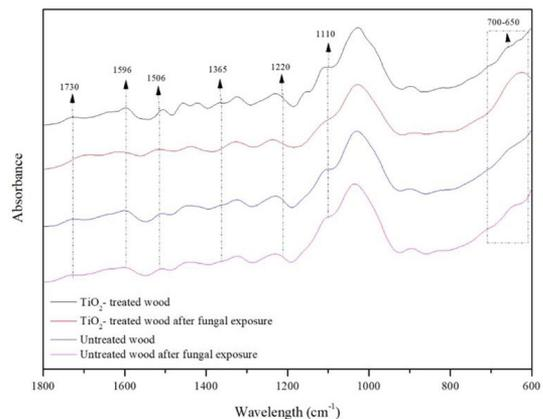
**Figure 2.** FT-IR spectra of untreated and TiO<sub>2</sub>-treated woods before and after the accelerated decay test.
