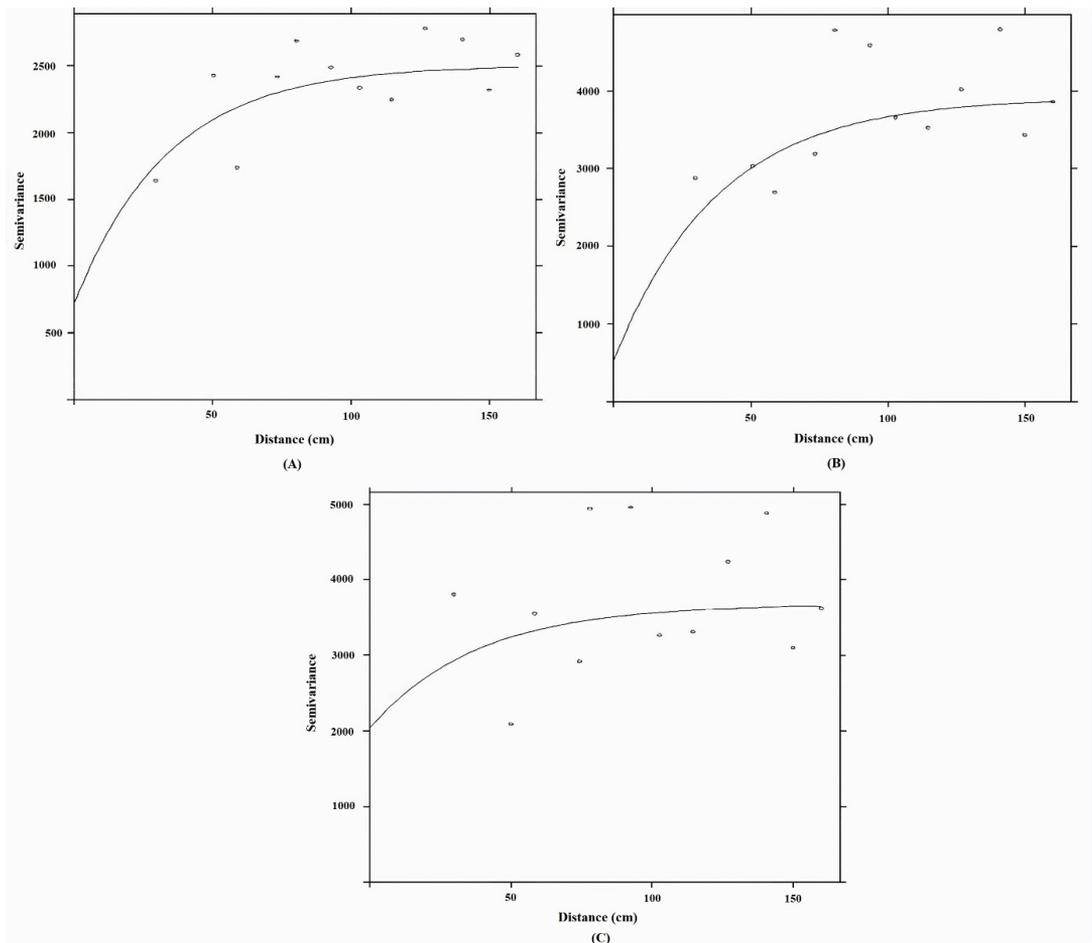
Figure 2. (A) Semivariogram of woodchip pile after 7 days of storage; (B) 30 days of storage; (C) 60 of storage.
