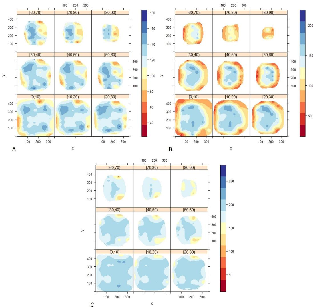
**Figure 3.** Graphical representation of woodpile moisture after 7 (A), 30 (B) and 60 days (C) of storage, showing variation in the moisture content at every 10 cm in height of the storage structure.
