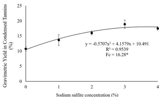
**Figure 4.** Gravimetric yield of condensed tannins as a function of sodium sulfite concentration. \*Significant using the *F*-test ( $p > 0.05$ ).
