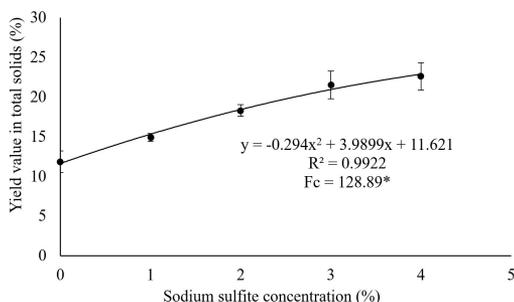
**Figure 2.** Yield of total solids as a function of sodium sulfite concentration. \*Significant using the *F*-test ( $p > 0.05$ ).
