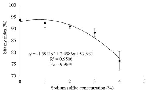
**Figure 3.** Stiasny index as a function of sodium sulfite concentration. <sup>ns</sup>Not significant using the *F*-test ( $p > 0.05$ ).
