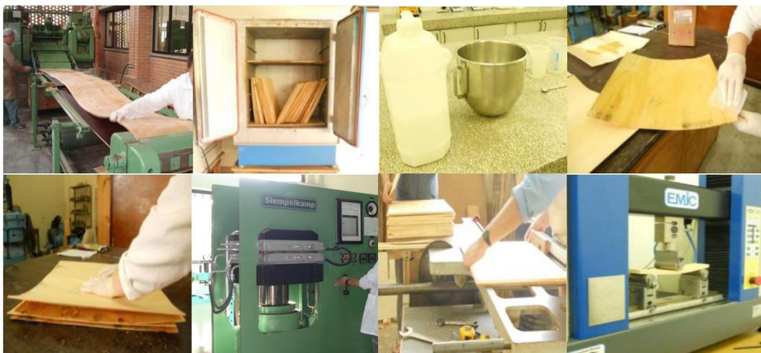
**Figure 1.** Stages of the manufacture and assessment of the plywood panels.
