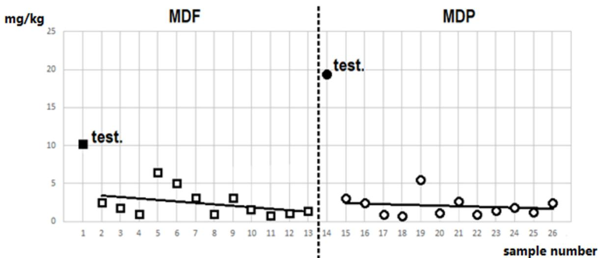
**Figure 3.** Dispersion values of formaldehyde emissions (mg/kg) found in the samples of MDF and MDP, including the equation of the trend line.
