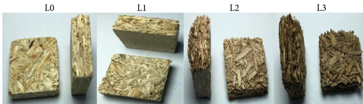
**Figure 2.** Samples of MDP medium density particleboards evaluated: new and degradation levels 1, 2 and 3.
