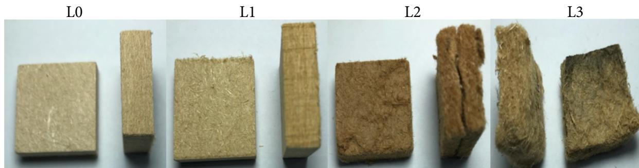
**Figure 1.** Samples of MDF medium density fiberboards evaluated: new and degradation levels 1, 2 and 3.
