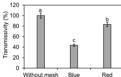
**Figure 2.** Solar radiation transmissivity (%) for the treatments Red mesh, blue mesh and no mesh. Different letters indicate significant differences (P<0.05) according to Tukey test.
