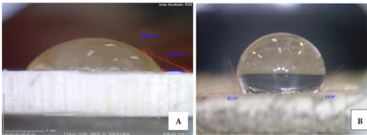
**Figure 2.** Contact angle between the water drop and the veneer surface in the wettability test. A - Untreated; B - CCA-C treated.
