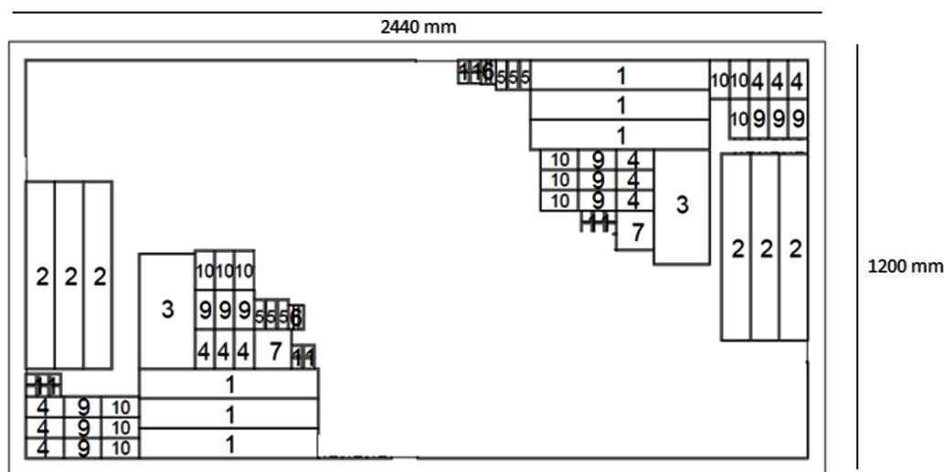
Figure 1. Cutting plane and plywood panels dimensions.
