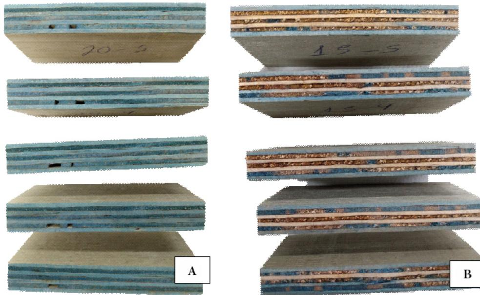
**Figure 3.** Penetration of the CCA-C preservative product into the treated plywood panels: A – pre- and B - post-pressing.
