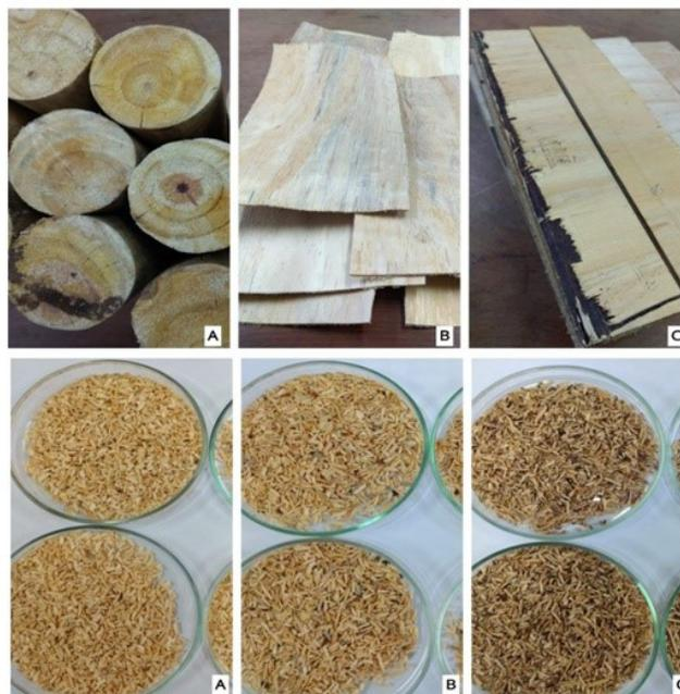
**Figure 1.** Types of waste collected and particles obtained after classification in sieves. A) Log core; B) Veneer clippings; C) Plywood cutting.
