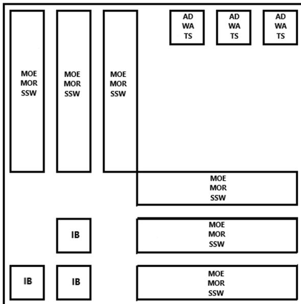
**Figure 2.** Sketch of the panels' specimens, where: AD = apparent density; MC= moisture content; WA= water absorption; IB= Internal bonding; TS= Thickness swelling; MOR = Modulus of rupture in static bending; MOE= Modulus of elasticity in static bending; SSW= Surface screw withdrawal.
