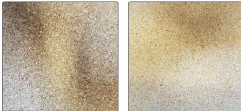
**Figure 1.** Squared panel with CCB treated wood particles (a) and untreated wood particles (b)
