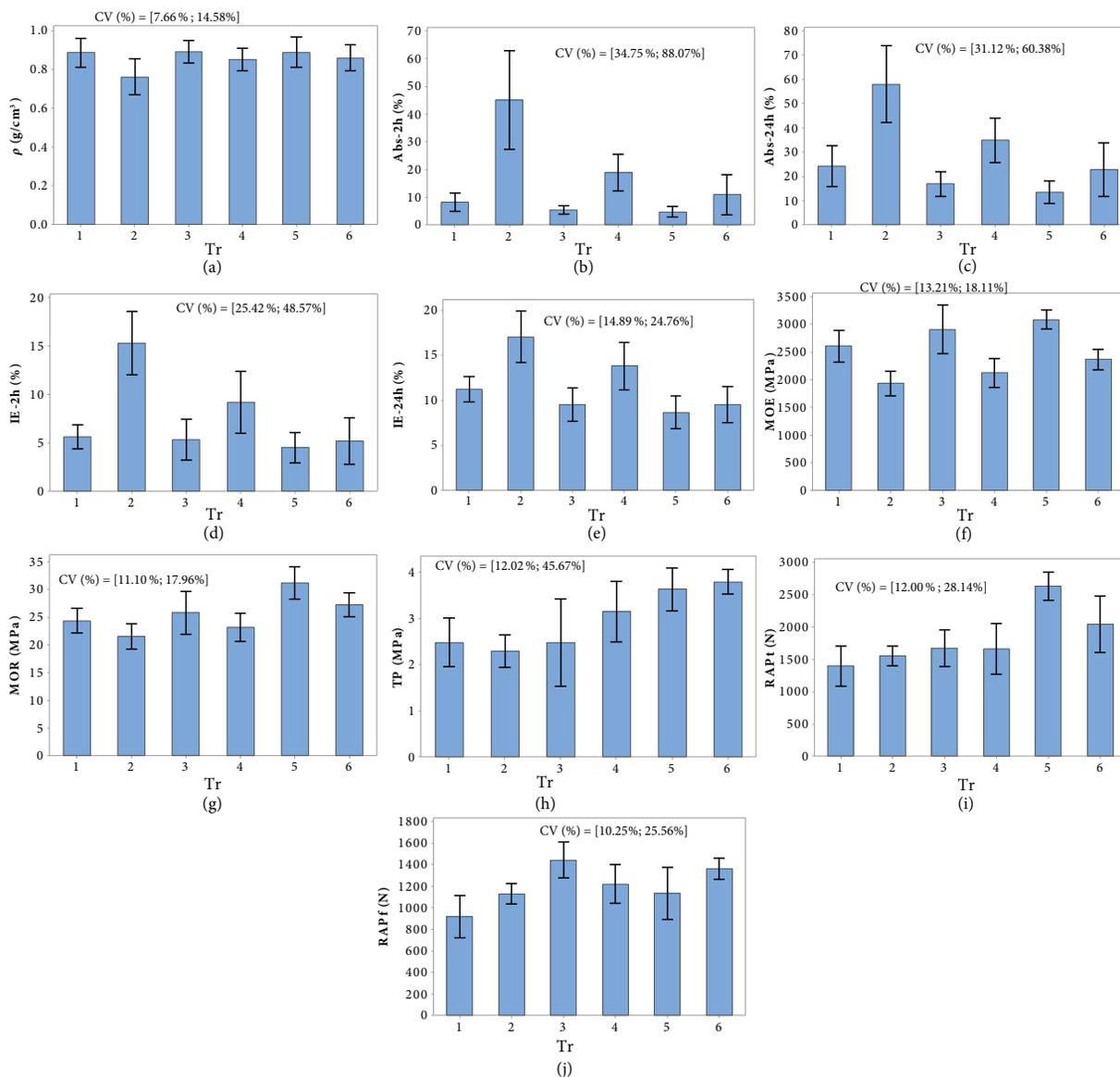
Where: density ( $\rho$ ); thickness swelling after 2 hours (IE-2h) and after 24 hours (IE-24h), water absorption after 2 hours (Abs-2h) and after 24 hours (Abs-24h), modulus of rupture (MOR), modulus of elasticity (MOE), normal tensile strength (TP), surface bolt pullout test (RAPf) and top bolt pullout test (RAPt).
